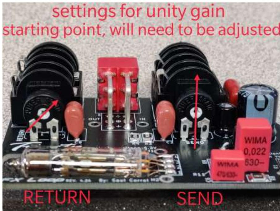
**Tube Fx Set-Up** If you have bench instruments, follow this procedure.
