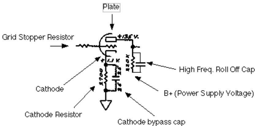
"Complete" typical tube preamp stage:
