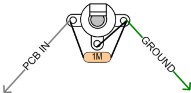
Connect the GREEN wire from the input jack ground lug to the preamp ground terminal lug on the enclosure. Connect GREEN ground wire from the volume control to the preamp enclosure ground lug also.
