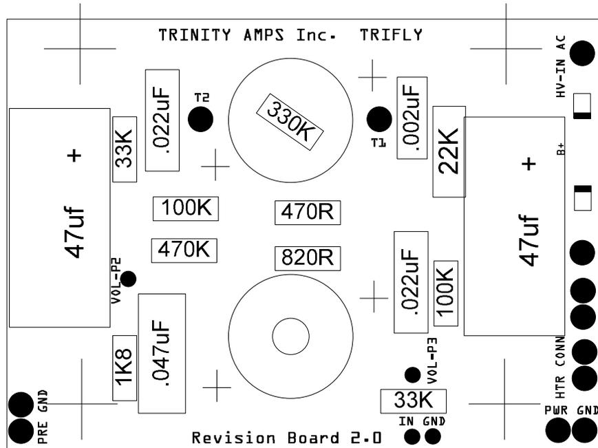
Then install the first 47 $\mu$ F filter capacitor.
