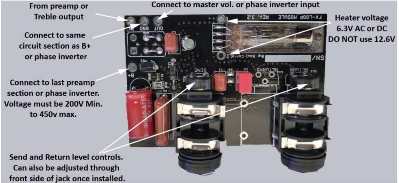
5. **HEATER VOLTAGE** This tube only works with 6.3V AC or DC. Do not use 12.6V! Wires for this voltage are connected to holes on sides of tube. If using 6.3VDC, positive can be on either side.
