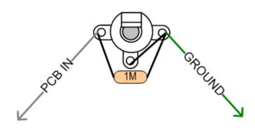
Connect the GREEN wire from the input jack ground lug to the preamp ground terminal lug on the enclosure. Connect GREEN ground wire from the volume control to the preamp enclosure ground lug also.
