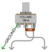
Solder a 3" GREEN lead to the ground lug. Solder a 3" White led to the IN lug (switched terminal).
