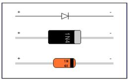
The cathode is marked by a line painted on the body of the diode. Diodes are labeled with their code in small print, and you may need a magnifying glass to read! The diagram below shows the orientation of the 1N4007UF diode.
