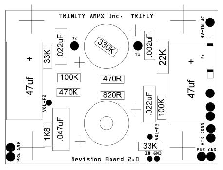
Then install the first  $47\mu F$  filter capacitor.
