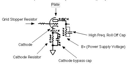
"Complete" typical tube preamp stage:
