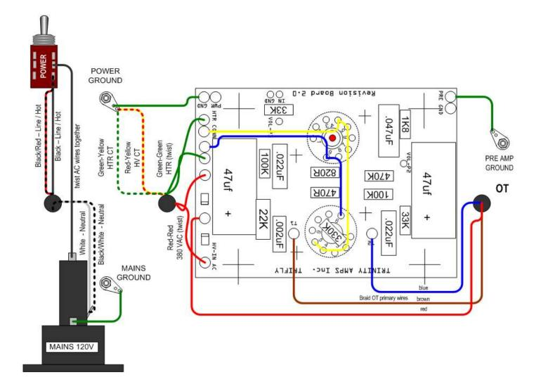
TriFly Heater and Power Supply Wiring
